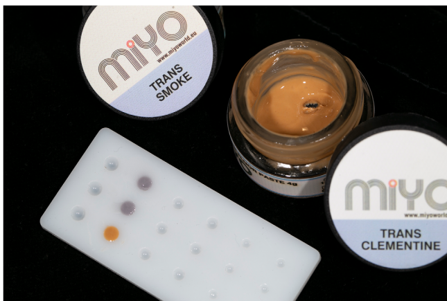
FIGURE 16 A silicone portioner (Smile Line, Saint-Imier, Switzerland) is used to prepare the given ceramic paste recipes by Matisse iOS App.
